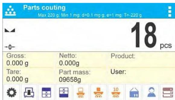
Stable measurement (stability pictogram displayed) can be printed. To do it press
