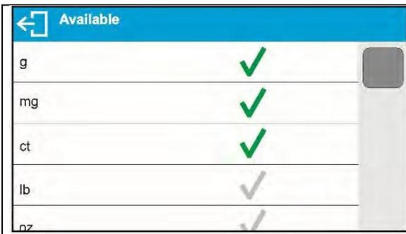
Units with parameter value set to <No ✓> option will not be accessible while operating the balance.
