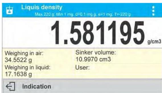
A report of the measurement can be printed through the attachment of printer to the balance. To print the report, press the
